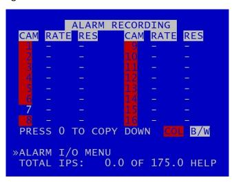
ALARM RECORDING is activated by the alarm inputs. This menu sets the alarm recording configuration.
