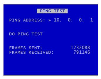
PING TEST menu enables the user to enter a destination IP address to send a network packet to testing connectivity.
