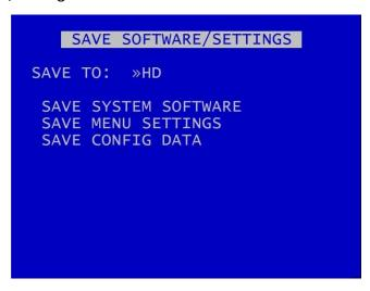
SAVE SOFTWARE/SETTINGS provides options for saving the current settings. The current software and settings will be written to the HD cartridge or SD card.
