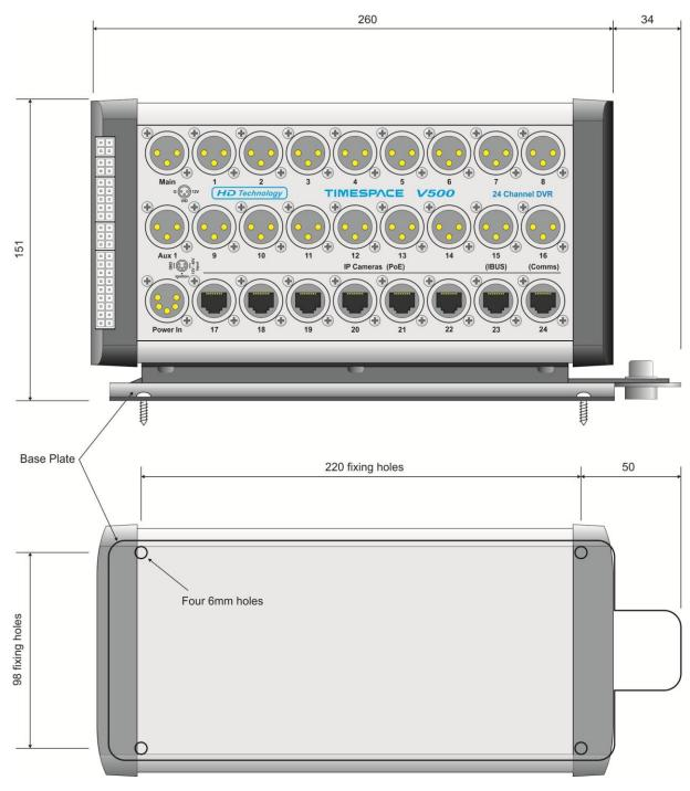
Figure 12 V500 Measurement Data
