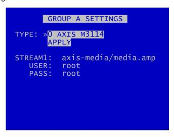
The GROUP SETTINGS menus A-D enable the user to select the type of camera to allocate to each group.
