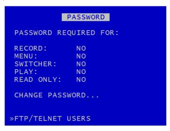
PASSWORD menu sets a password to restrict user access to five key areas of the system. A read-only access can be set that allows files to be viewed and limited features to be used. For each area, select YES/NO.
