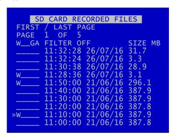
The SD CARD RECORDED FILES menu lists the files recorded on the SD card.
