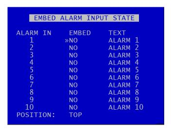
The EMBED ALARM INPUT STATE menu configures options for adding text to recorded images.
