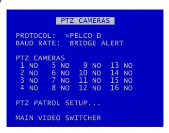
PTZ CAMERAS menu allows control over a Pan, Tilt, Zoom camera when connected to the V500's serial port. An RS232-to-RS485 convertor will be required – example convertor; **EXTERNAL LINK**, Farnell code; 1683075.
