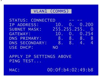
The VLAN 1 menu allows the user to change the parameters of the VLAN 1 system.
