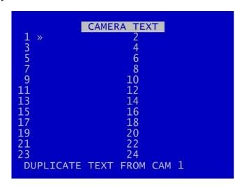
Individual text for each camera can be inserted above the timestamp. This text, along with timestamp, will be shown on recorded images.
