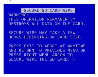
SECURE SD CARD WIPE will permanently delete all recording files on the SD card. This should only be used if files need to be completely destroyed. NO files will be able to be recovered. A final warning message will appear before this function is carried out. Pressing Menu Exit will abort.
