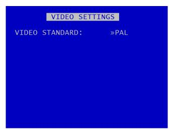
VIDEO SETTINGS menu controls the video standard, i.e. whether the unit is to operate with PAL or NTSC cameras.
