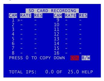
SD CARD RECORDING menu - The V500 can be configured to record up to 25 images per second (IPS) to the SD card in addition to the primary images per second being recorded to the cartridge. All additional data e.g. audio and GPS are also included within the SD recorded files.
