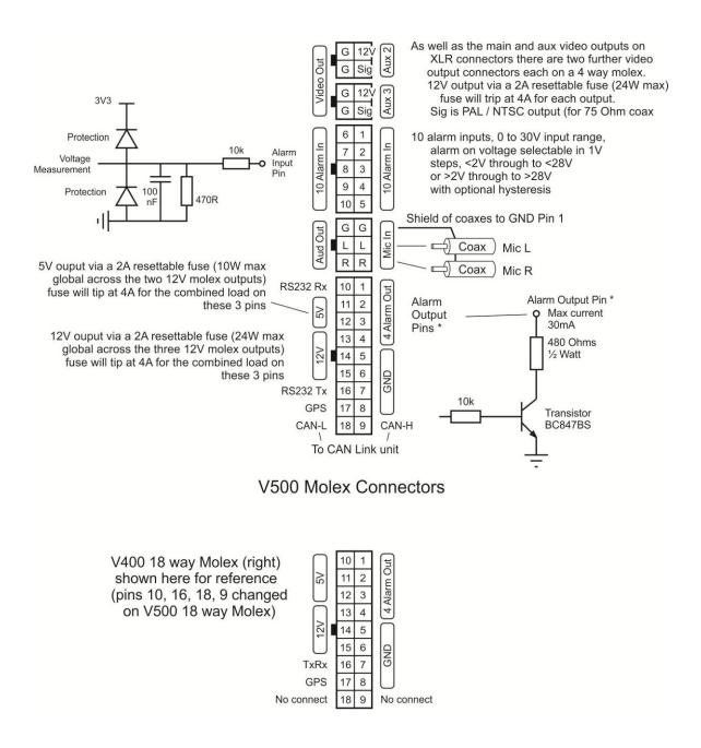
Figure 11 V500 Molex End Panel Connectors
