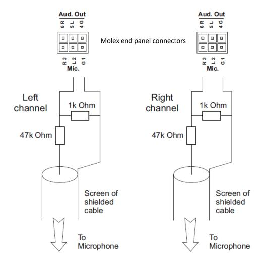
Figure 16 Wiring a line level microphone
