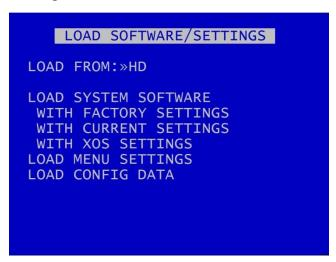
LOAD SOFTWARE/SETTINGS menu provides options for loading new/upgraded software and/or settings. An .XOS file should be copied onto the cartridge or SD card using a PC then inserted into the V500.
