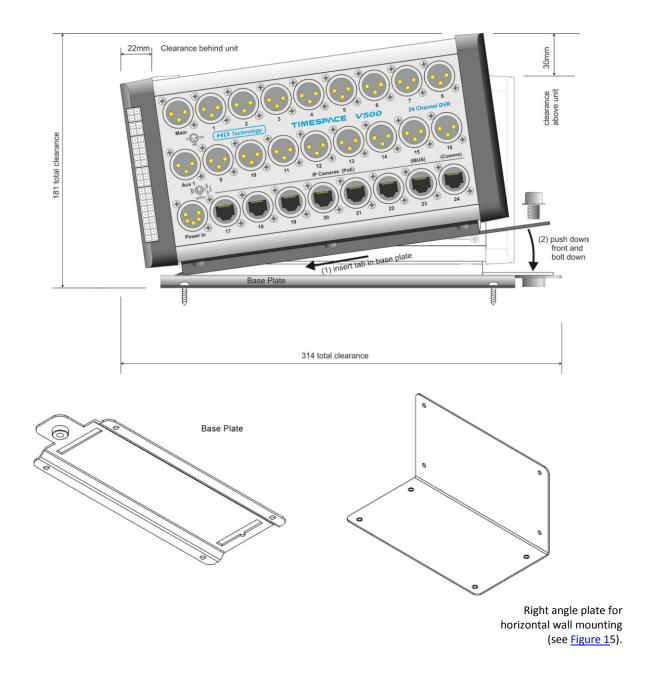
Figure 14 Mounting Plates
