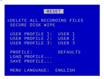
Three User Profiles can be configured with different settings for different uses or recording modes. This gives the user an easy way of quickly switching between types of recording required without having to setup the V500 each time. Each profile can be named individually.
