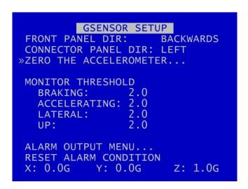
GSENSOR SETUP menu displays the GSensor configuration. The GSensor is calibrated as part of the manufacturing process in a controlled environment and should not require calibration during the installation process.
