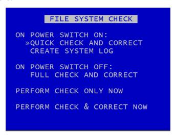
FILE SYSTEM CHECK menu configures whether the file system is checked (and possibly corrected) at power up and also if a system log is created.
