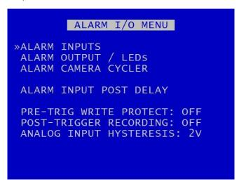
Alarm Inputs and Outputs can be configured as per the <u>ALARM INPUTS/OUTPUTS</u> menu in settings for <u>ALARM RECORDING</u>.
