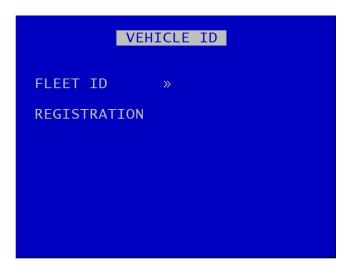
This menu page allows entry of the vehicle's fleet ID number and registration number. This is recorded in system and health logs and makes it easier when using LANLink to identify the vehicle in which the recorder is fitted.
