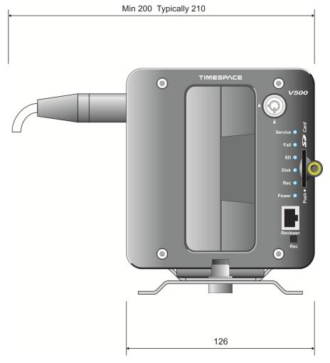
Figure 13 V500 Front Panel Measurement Data
