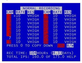
NORMAL RECORDING sets the normal recording configuration. Recording is activated by pressing the record button on the <u>front of the V500</u> or the <u>Reviewer</u>. The V500 is also set to default record on power-up.
