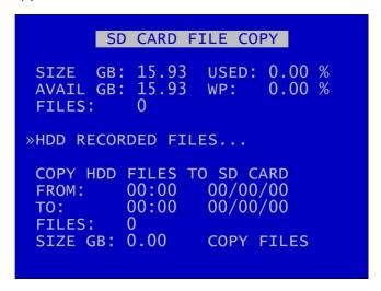
SD CARD FILE COPY is used to copy recorded files from the V500 cartridge to the SD card. A link to the main cartridge HDD files give quick access to see what is on the cartridge. Some SD statistics are given to aid in the select process e.g. size and capacity used.
