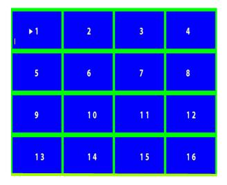
MULTI CAMERA SETUP configures which of the analogue cameras 1-16 are to be displayed simultaneously. Each tile can be set to display a sixteenth view of a camera. If the same camera number is set to four tiles in a square then a quarter view will be shown.
