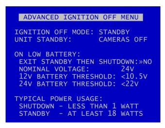
ADVANCED IGNITION OFF MENU provides options for the unit to be set to SHUTDOWN or STANDBY mode when ignition is off.
