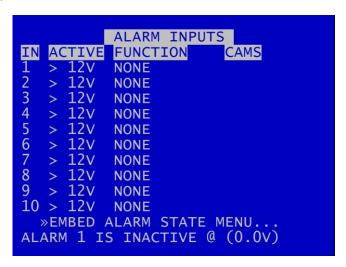
ALARM INPUTS menu sets the alarm inputs to be ACTIVE or INACTIVE. If an alarm input number is highlighted with a white background, this indicates its current state is active. No highlight indicates the state is inactive.
