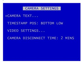
CAMERA SETTINGS menu configures the <u>CAMERA TEXT</u> labels, timestamp position, <u>VIDEO SETTINGS</u> and camera disconnect time.
