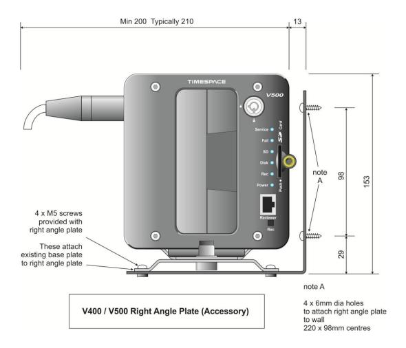
Figure 15 Right Angle Mounting Plate details
