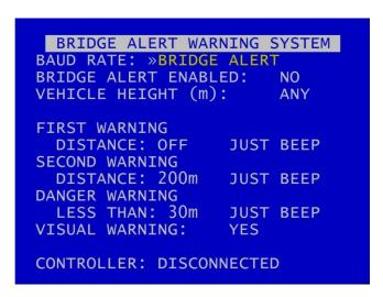
The BRIDGE ALERT WARNING SYSTEM menu enables BRIDGE ALERT and configures its settings.
