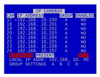
The IP CAMERAS menu configures settings for the 8 IP camera inputs supported by the V500 unit. Additional support for installing IP Cameras can be obtained by emailing  $\underbrace{ \text{support@tspace.co.uk} }_{\text{co.uk}}.$
