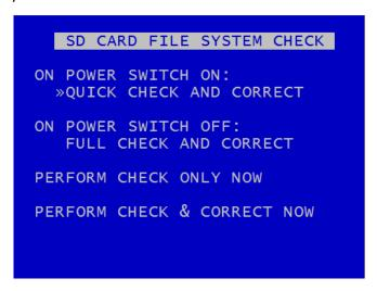
SD CARD FILE SYSTEM CHECK menu configures whether the file system is checked and/or corrected at power-up and whether a system log is created.
