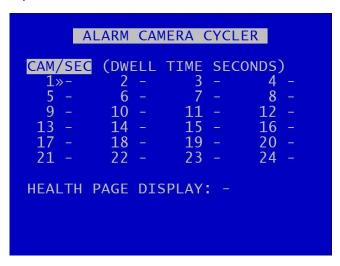
The ALARM CAMERA CYCLER menu configures the options for the V500 to automatically switch between cameras and the <u>Health Page</u>.
