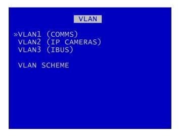
In order to allocate LAN resources, physical ports 17-24 on the DVR (see diagram for <u>V500 side panel</u>) can be partitioned by means of VLAN (Virtual LAN) tagging.
