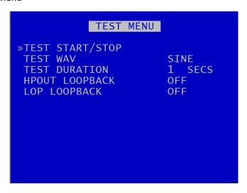
The AUDIO TEST MENU sets the parameters for carrying out an audio test.
