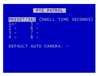
The PTZ PATROL menu configures the PTZ cameras to switch between preset positions as set by the user. This is similar to setting up the <u>Main Video Switcher</u>.
