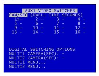
AUX VIDEO SWITCHER configures the settings for the three auxiliary (secondary) video outputs, AUX1-3.
