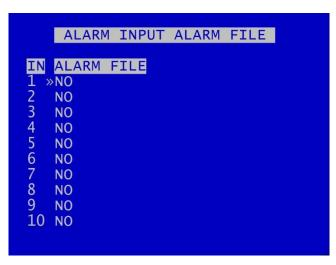
The Alarm Input Alarm File feature provides an option for files to be marked as ALARM recordings even if recording in NORMAL or TIMER RECORDING modes.
