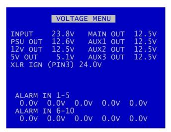
VOLTAGE MENU page displays the current Voltage supply, broken down into various sections e.g. Main video output, Alarm Inputs etc.
