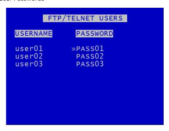
FTP/TELNET USERS menu gives the option to have three different passwords to access the V500 via FTP/TELNET.
