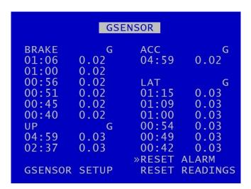
GSENSOR menu configures settings for the V500's built-in accelerometer.
