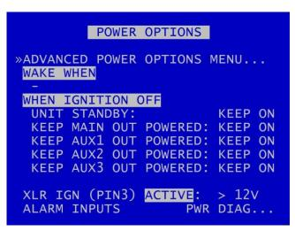
POWER OPTIONS menu configures the behaviour of the V500 when power is applied, when power is removed and when an input trigger is detected.
