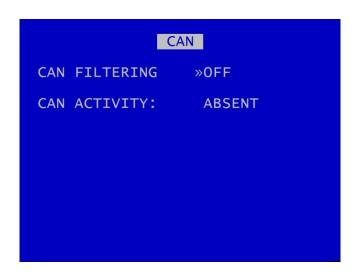
Timespace has developed vehicle CAN (Controller Area Network) reporting system. A secure CAN interface enables the DVR to record CAN data and download vehicle CAN information via the vehicle depot's Wifi/LANLink system.
