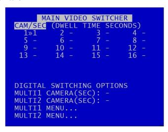
MAIN VIDEO SWITCHER menu controls the video output on the Main Switcher.
