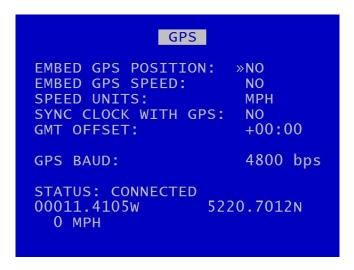
The GPS menu is the setup menu for the Global Positioning System serial connection.
