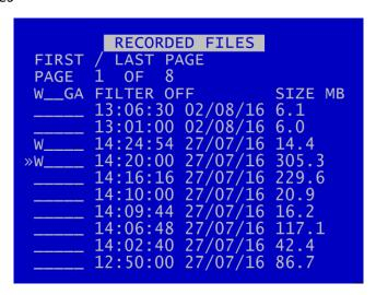
RECORDED FILES menu lists the recorded files on the HDD and allows the user to select a file to play or to change the write-protect state of a file.
