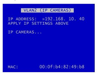
The VLAN 2 menu allows the user to change the IP address of the VLAN2 port.
