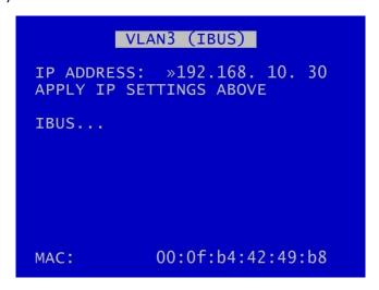
The VLAN3 menu allows the user to change the IP address of the VLAN3 port.
