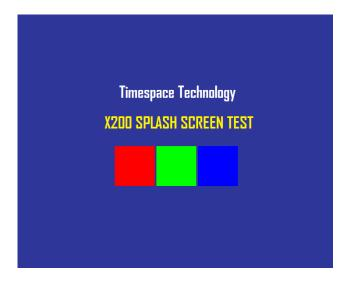
Once in the correct format (using the Timespace conversion tool), the image is placed on the V500 cartridge, named; Splash.ext. Once configured in the menu, the Splash Screen will be read from the disk and displayed.
