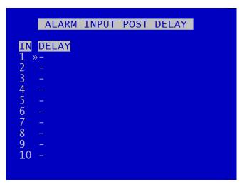
ALARM INPUT POST DELAY menu controls the number of seconds for which the alarm state is held once the alarm input has changed state.
