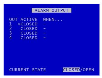
ALARM OUTPUT menu sets the conditions for the Alarm outputs. This determines whether the V500 alarm output goes closed (pull to GND) or open circuit when any of the set conditions are met.
