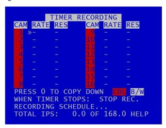
TIMER RECORDING sets daily on/off timers to provide timed recording. This menu sets the recording configuration and the times. During TIMER RECORDING the settings in this menu apply.
