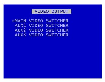
VIDEO OUTPUT menu controls the automatic switching and dwell time of cameras on the four video outputs:
