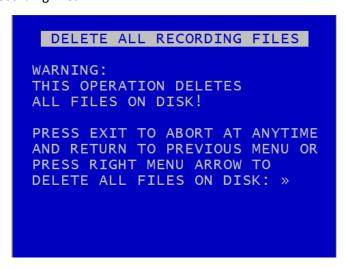
DELETE ALL RECORDING FILES – will remove all recordings from the hard disk, <u>including write-protected files</u>.
