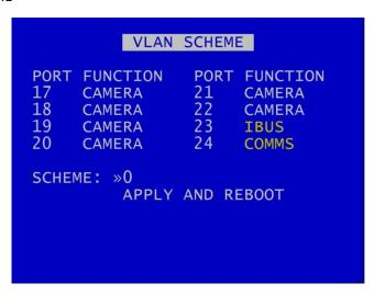
The VLAN SCHEME menu lists the various options for VLAN Connections.
