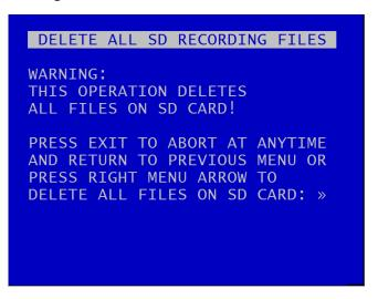
DELETE ALL SD RECORDING FILES will remove all recordings from the SD card including write-protected files. Only do this if you want to completely remove all recordings – there is NO undo option. Press the <u>right menu button</u> to go to a warning screening, press right again to carry out this action. Pressing <u>Menu Exit</u> will abort this procedure.
