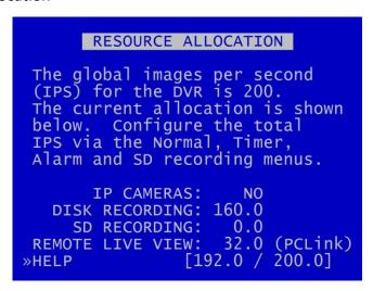
The RESOURCE ALLOCATION page provides details of the images per second (IPS) allocation as currently configured on the V500. The IPS allocation values shown indicate the quantity of IPS currently assigned to IP Cameras, Disk Recording, SD Recording and Remote Live View.
