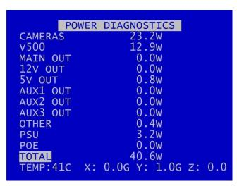
POWER DIAGNOSTICS page displays the current power consumption, broken down into various sections e.g. Cameras, GPS.
