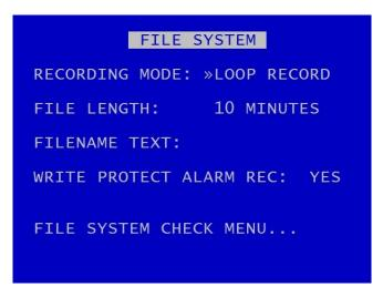
FILE SYSTEM MENU Sets the parameters of the file system and how files are laid to disk.
