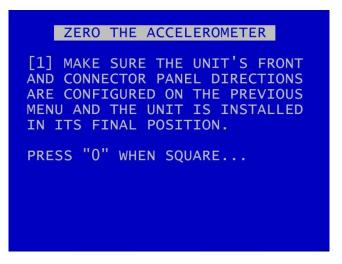
Once the V500 is installed in its final operating position, the GSensor readings must be zeroed by entering "0" when on the ZERO THE ACCELEROMETER screen.
