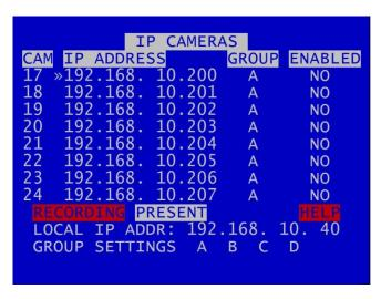
The IP CAMERAS menu configures settings for the 8 IP camera inputs supported by the V500 unit. Refer to IP CAMERAS menu section under MAIN MENU option.
