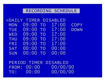
A RECORDING SCHEDULE can be set. This can be used e.g. to record between a start date and end date. If both DAILY TIMES and PERIOD TIMES are selected, the V500 will record only in the period and also only in the daily times shown.
